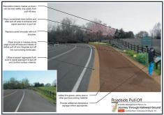
Figure 153 Existing "last holdup" historic marker near the Raulston Stand (top) and shoulder treatment and flush curbs that would make the pull-off safer and more usable
